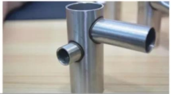
360 degree no dead seam weld
