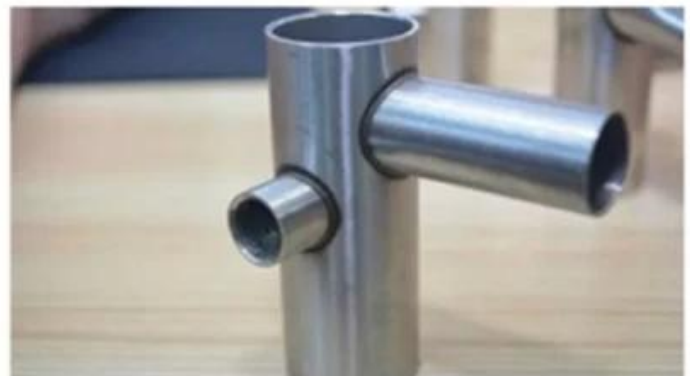
360 degree no dead seam weld
