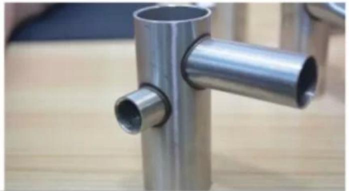
360 degree no dead seam weld
