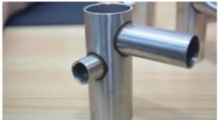
360 degree no dead seam weld
