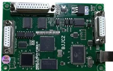
Laser control card enables real-time control of scan system and lasers over a standard USB host interface. Customers can integrate complete machinery easily over the laser control card due to its compactness and I/O capabilities. Fast response times and short execution cycle times make the EzCad Card perfectly suitable for high performance applications. It can load marking file via a removable MMC memory card.
