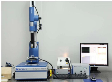
TRIOPTICS OptiSpheric 2000 AF ---Testing EFL、R、Centering Error、Wedge Angle、BFL、MTF
