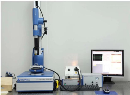
TRIOPTICS OptiSpheric 2000 AF ---Testing EFL、R、Centering Error、Wedge Angle、BFL、MTF
