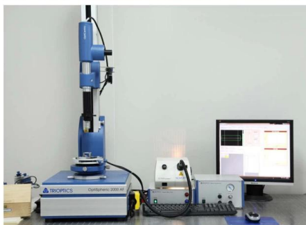
TRIOPTICS OptiSpheric 2000 AF ---Testing EFL、R、Centering Error、Wedge Angle、BFL、MTF
