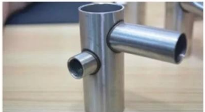
360 degree no dead seam weld
