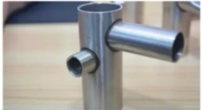
360 degree no dead seam weld
