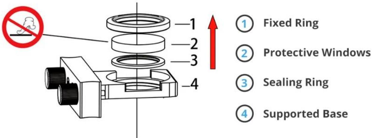
**NOTICE:** 1—3 Parts Should be taken out in the direction of the arrow, otherwise these parts will be damaged.
