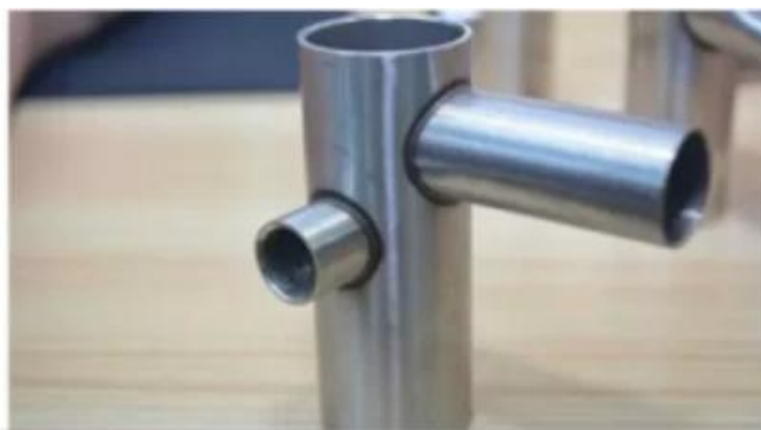
360 degree no dead seam weld
