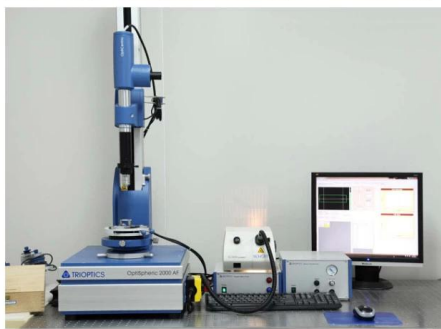
TRIOPTICS OptiSpheric 2000 AF ---Testing EFL, R, Centering Error, Wedge Angle, BFL, MTF
