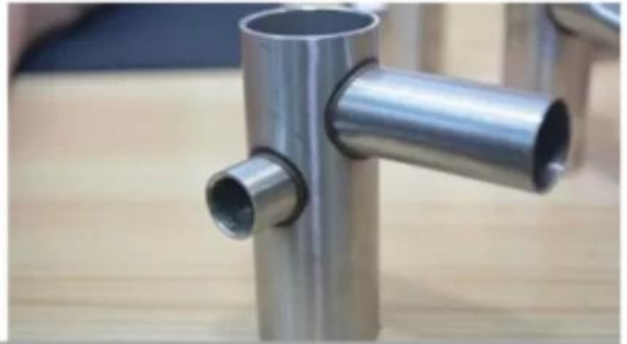
360 degree no dead seam weld
