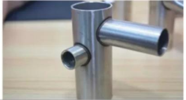
360 degree no dead seam weld
